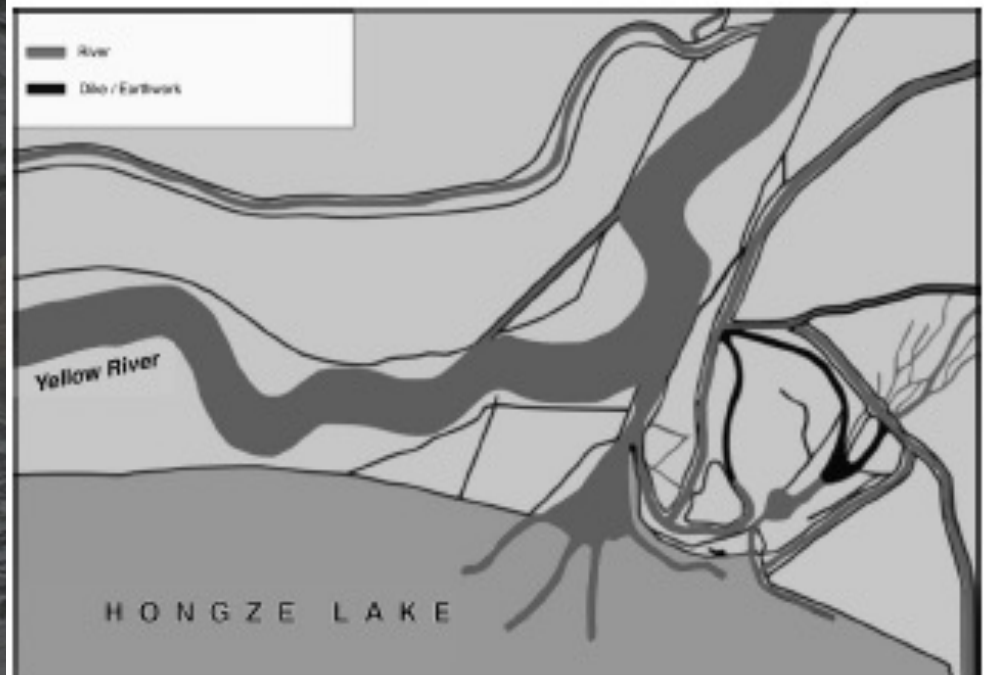
FIGURE 4.18 The Evolution of Hydrological Architecture around the Qingkou Confluence. The major features of the confluence of Hongze Lake, the Yellow River, and the Grand Canal were the Qingkou passage, Gaojiayan Dam, and various watercourses. Although construction of the Qingkou system began in the Ming era, it did not reach full buildout until the eighteenth century. These images depict the Qingkou confluence at (a) prior to the fourteenth century, (b) 1776, and (c) 1854. Based on Zhang et al., "Qingkou Complex,"
